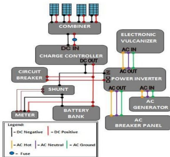
Fig. 2: Schematic diagram of solar power electronic vulcanizing equipment
